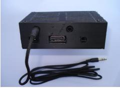
And one for Tx IQ connection, it should be connected to "TO LINE OUT" SDR1000 input and to the left upper side connection of Pi SDR IQ Plus
