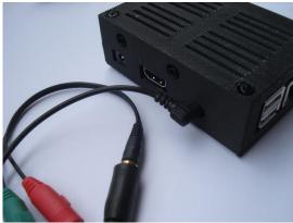
NOTE: Most PC headsets (if they have a 4 pin, 3.5mm TRRS connector) use the CTIA standard therefore will not work when plugged directly into the Pi-SDR IQ Plus. An OMTP to CTIA adapter cable is provided with the Pi-SDR along with a 4 pin TRRS splitter cable for headsets with separate MIC / PHONE TRS 3.5mm connectors.
