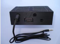
And one for Tx IQ connection, it should be connected to IQ-IN TX input of RS-HFIQ and to the left upper side connection of Pi SDR IQ Plus
