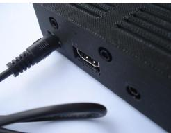
The user provided power supply needs to have three requirements, first to have a USB connector to connect with the provided power cable, second to be rated 5V 2.5Amp and finally to be 'quiet' in terms of electrical noise effects.
